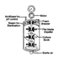
ii. Sparged stirred-tank bioreactor through which sterile air bubbles are sparged.
