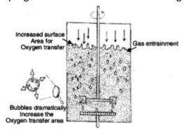
One of the most commonly used bioreactors is of stirring type.
